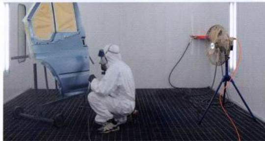
Ventilation in painted booths and explosion-proof areas that are not equipped with ventilation facilities, and air blowing to prevent heat stroke. In addition, it can be used for drying product paints.
